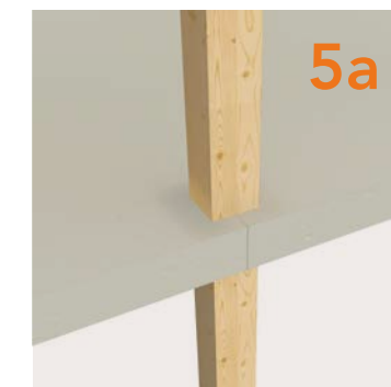
The columns for the next storey are fitted
