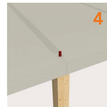
The elements are friction-fitted and the joints are sealed
