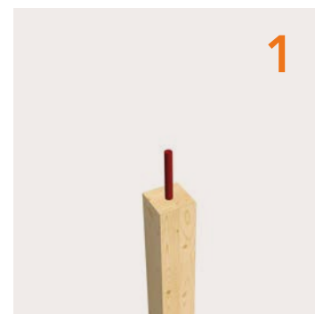
The facade column is put into position, with a steel connector ready fitted
